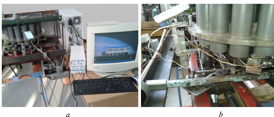
Fig. 4 – Apparatus for determining the distribution device permutation time: 1 – distribution device; 2 – reception tube; 3 – acquisition data board; 4 – LED Infrared; 5 – infrared photo transistor; 6 – micro-contact; 7 – shutter.
