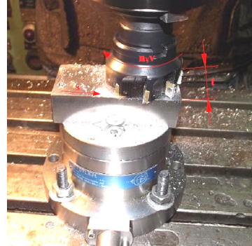
Fig. 5 – Processing by symmetrical and incomplete cut-up face milling.
