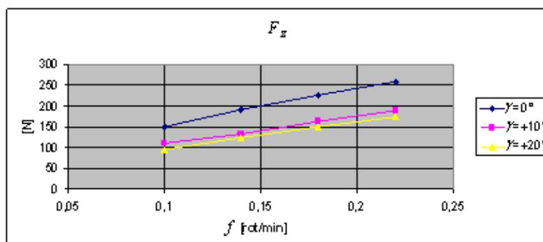
Fig. 12 – Evolution of cutting force  $F_c$  depending on rake angle values for different feed rates.
