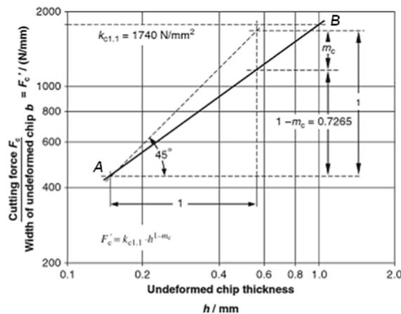
Fig. 6 – Graphical determination of characteristic values  $k_{c1.1}$  and  $m_c$  (Klocke, 2011).
