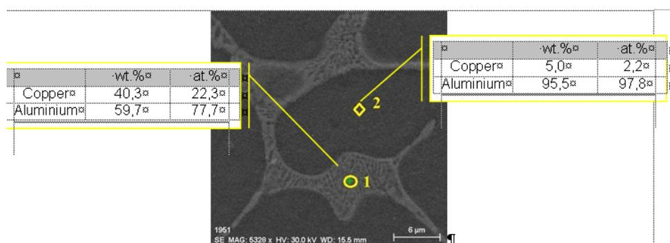
Fig. 3 – The elemental chemical analysis in two points.
