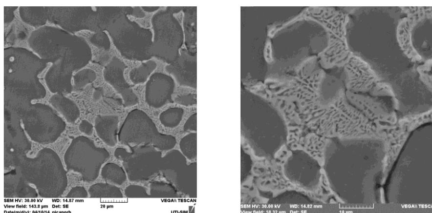
Fig. 2 – The electron microscopy of CuAl11 alloy.
