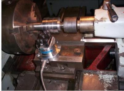
Fig. 10 – Measuring the resultant force and its components.
