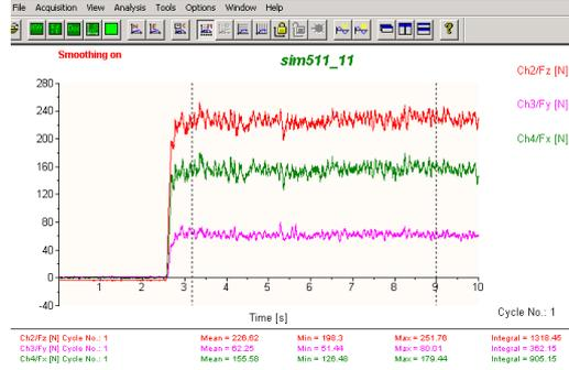
Fig. 11 – Registration of the resulting cutting force components.
