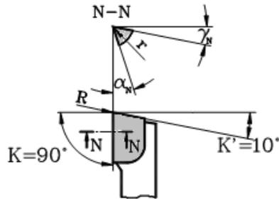
Fig. 7 – Geometric features of the utilized cutting tool.
