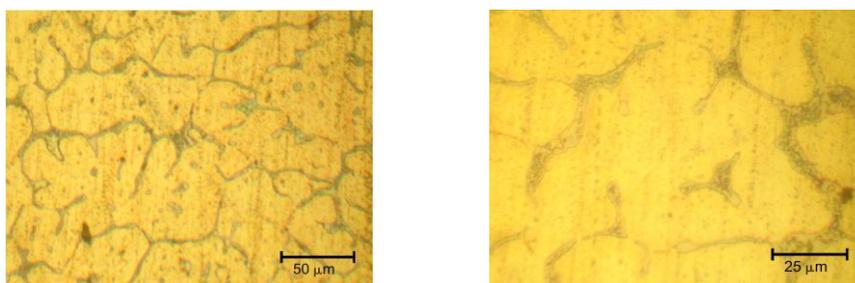
Fig. 1 – Microstructure of alloy AlCu11 (optical microscopy).
