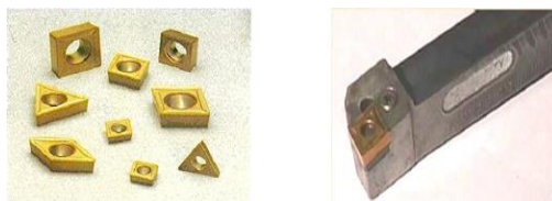
Fig. 2 – Indexable inserts (a); Clamped-tip tool (b).
