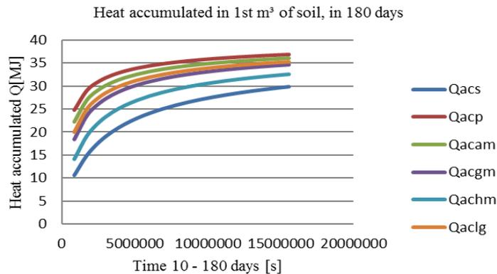
Fig. 10 – Heat accumulated underground for  $x = 1$ , (1 m<sup>3</sup>), in time, from day 10 to day 180, for a temperature of heat transfer fluid of 30°C.
