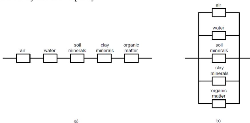
Fig. 1 – Soil particles arrangement for estimating average soil thermal conductivity:
