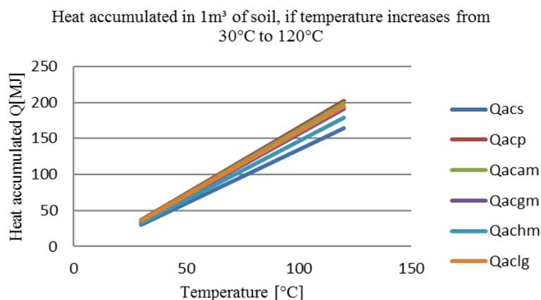
Fig. 8 – Heat accumulated underground if temperature of heat transfer fluid would increase from 30°C to 120°C.
