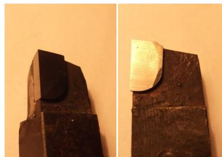
Fig. 2 – Geometric features of the utilized cutting tool. Fig. 3 – Cutting tool for  $\gamma_N = 0^\circ$  ( $\delta_N = 90^\circ$ ) and for  $\gamma_N = +10^\circ$  ( $\delta_N = 80^\circ$ ).
