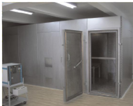
Fig. 2 – Access door for an anechoic chamber.
