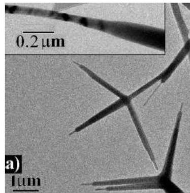
Fig. 2 – TEM images of nanowires (Roy *et al.*, 2003) growing out of a tetrapod leg, inset shows a magnified image of the nanowire – tetrapod leg.
