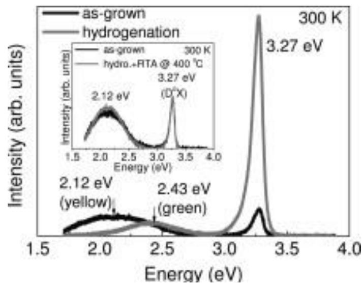
Fig. 5 – Photoluminescence spectra at room temperature of the as-grown and the hydrogenated *n*-ZnO bulk samples reported in (Kim *et al.*, 2011). The inset shows the PL spectra for annealing at 400°C of the hydrogenated sample.
