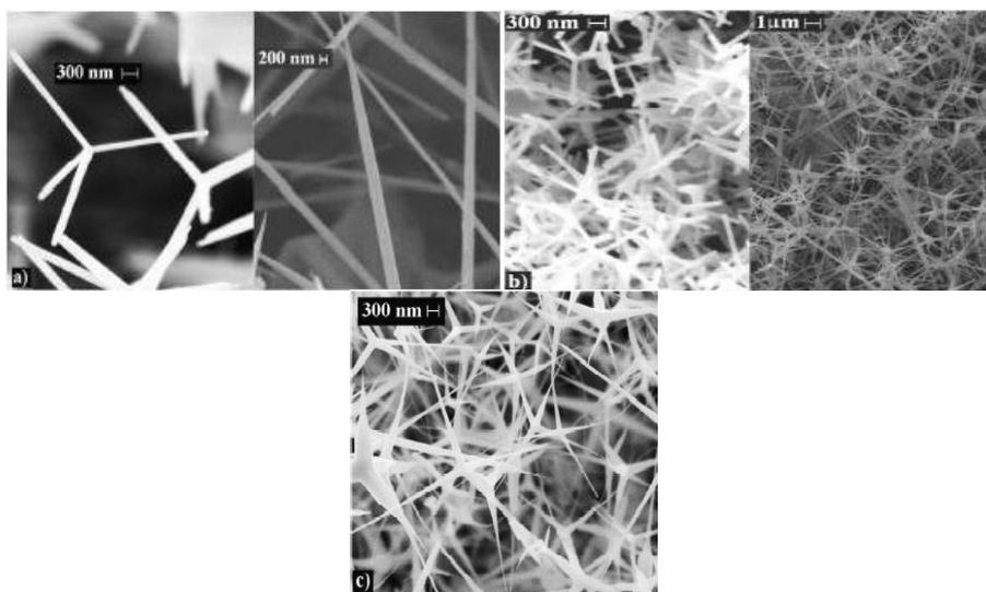
Fig. 1 – SEM images from ZnO nanostructures (Roy *et al.*, 2003): (a) tetrapods (left) and rods (right) obtained in the air; (b) small tetrapods (left) and mixture of tetrapods and wires right obtained in dry argon flow; (c) mixture of tetrapods and wires obtained in humid argon flow.
