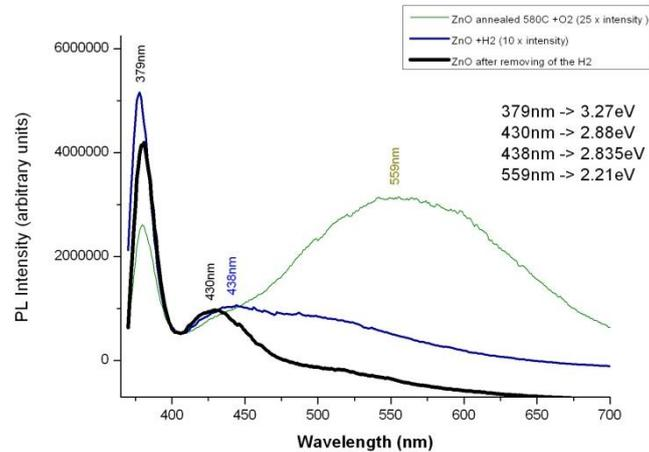
Fig. 6 – Photoluminescence spectra for annealing at 580°C and activated in O<sub>2</sub> sample, in presence of and after outgassing the H<sub>2</sub> samples.
