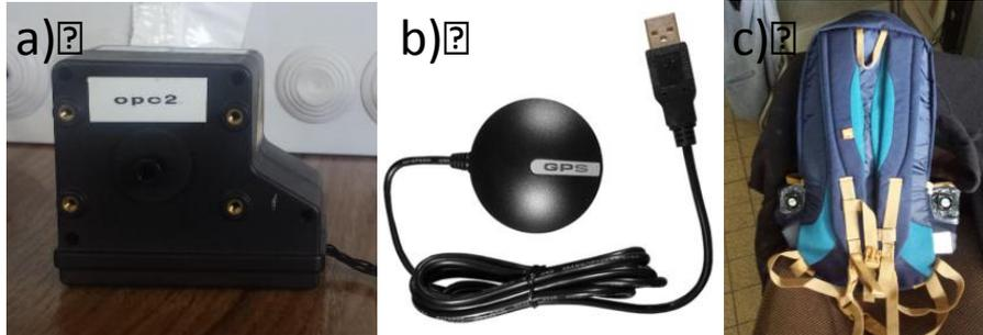
Fig. 1 – Illustration of the *a)* OPC-N2 Alphasense, *b)* GPS – model BU-353 and *c)* Backpack set up with two OPC mounted in the side pockets.
